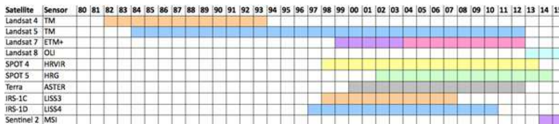
Figure 2: Timeline of currently available and scheduled future (Landsat 8, Sentinel 2) optical satellite data with at least one band in the short wave infra-red of at least 30 m spatial resolution. The change in the colour for ETM+ indicates the scan-line-corrector failure in 2003.
